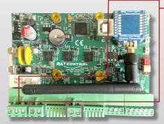
Integrated interface for LoRa WL Module Code: 0449, WLM-LORA-TIV50-433-A (module available for additional payment)
