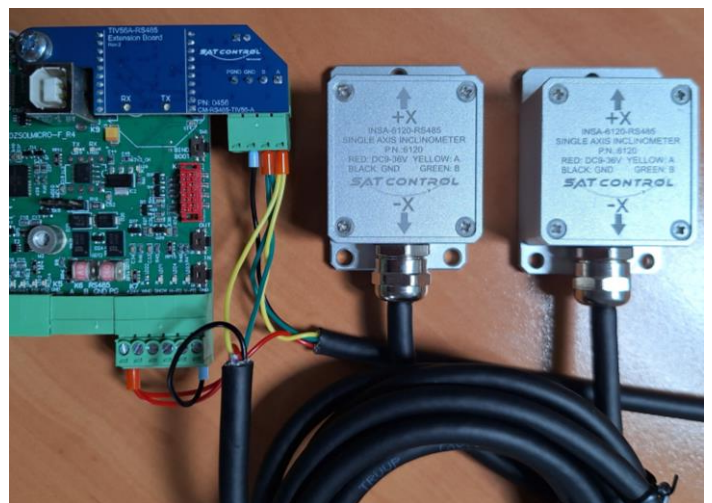
Example of connection of single sensor on internal RS485 port (left), and two sensors on external RS485 extension board (right)
