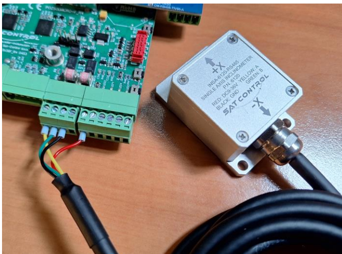
Example of connection of single sensor on internal RS485 port (left), and two sensors on external RS485 extension board (right)
