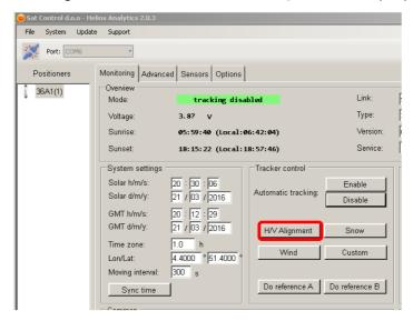
H/V aligment: Adjust motor to total horizontal position.
