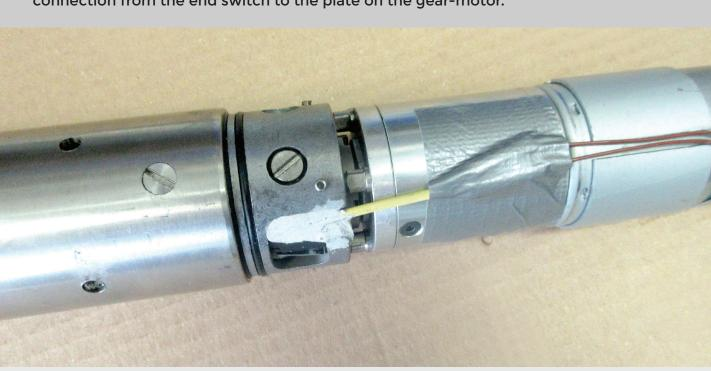
19. Use adhesive tape to fix the wires so that they fit in the notch, thus making a straight connection from the end switch to the plate on the gear-motor.
