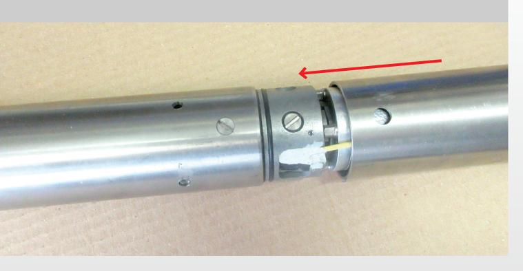
22. Screw the three bolts on the motor cover.
