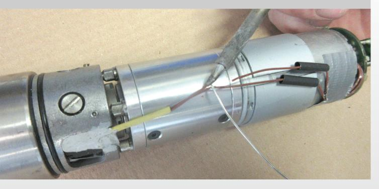
18. Place the shrink sleeves over the soldered part. Heat the sleeves with a high-temperature burner so that they shrink to fit the wires.
