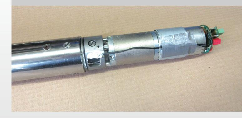
4. Cut off the cables that connect the motor with the end switch.
